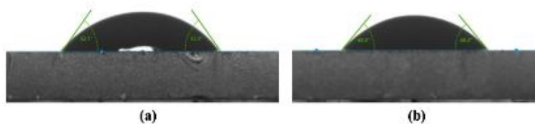
Fig 6.20: Contact angles of (a) GOPE and (b) sGOPE
